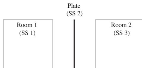
Fig. 4. Schematic of two statistical acoustic volumes separated by a statistical flat plate (SS J represents subsystem J).
